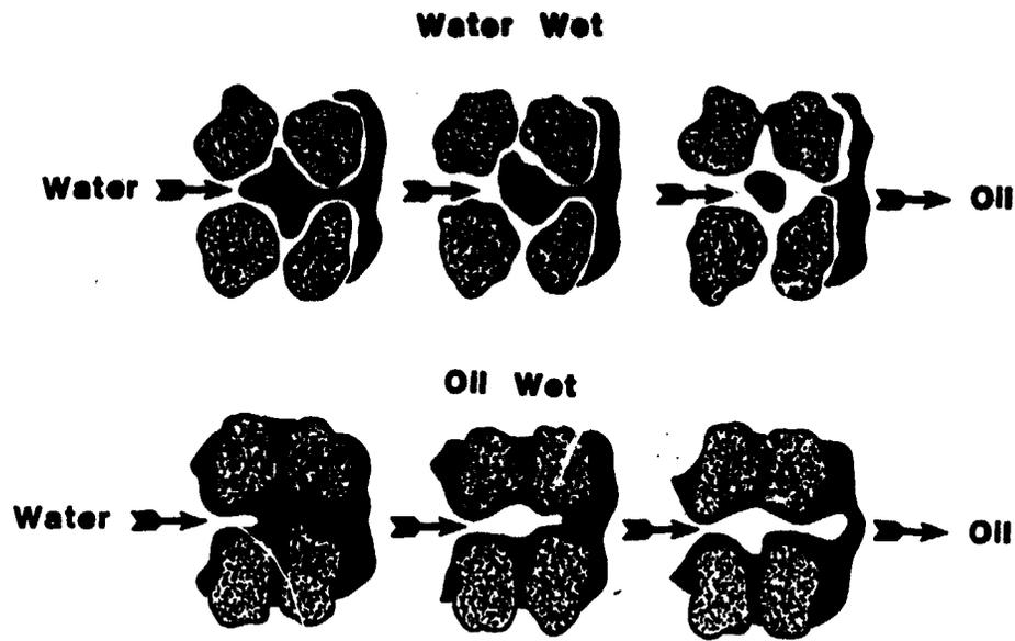
Fig. : 1 FLUID FLOW IN WATER - WET AND OIL - WET ROCK
